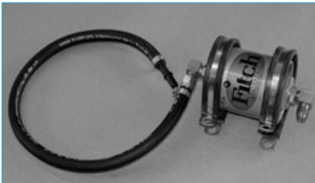
*The install kit also comes with a pair of clamps to hold the canister in place. We found a good spot inside the engine bay and used the two 90-degree fittings. Two holes needed to be drilled in the fender skirt to mount the canister. All the hardware you need is included with the install kit. It took us about a half-hour to install the canister – benefits to your engine begin immediately.*
