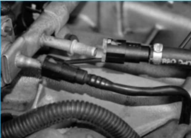
*The install kit for our Cherokee included these stock-style fuel clips. The line snapped right into place on the fuel injection rail. Fitch recommends installing the system as close to the engine as possible.*
